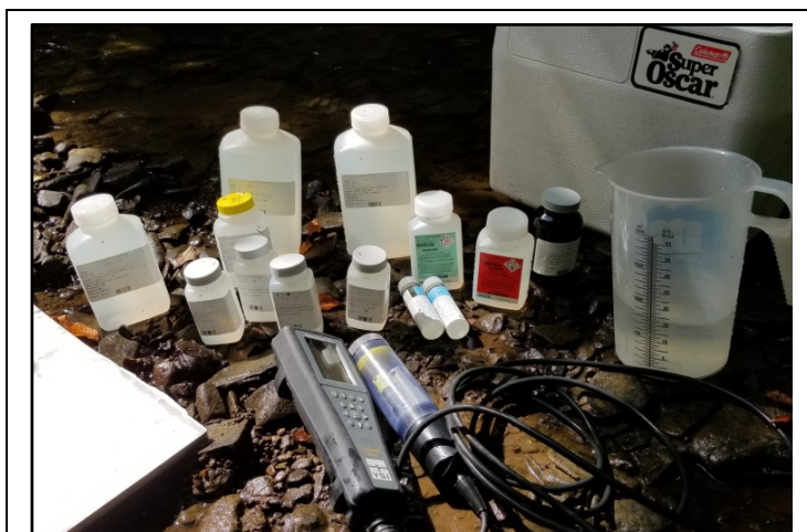
Figure 2. Materials used for sample collection, including collection beaker, sample bottles, YSI sonde for field parameter measurements.
